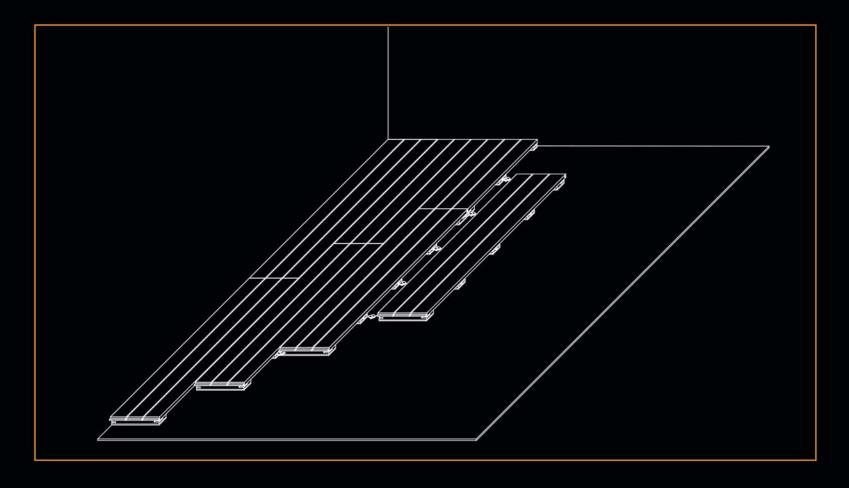
For a more aesthetic look, the *Trendy Dreck Floor* modules are designed to allow an English laying (butt joints staggered between the rows)
